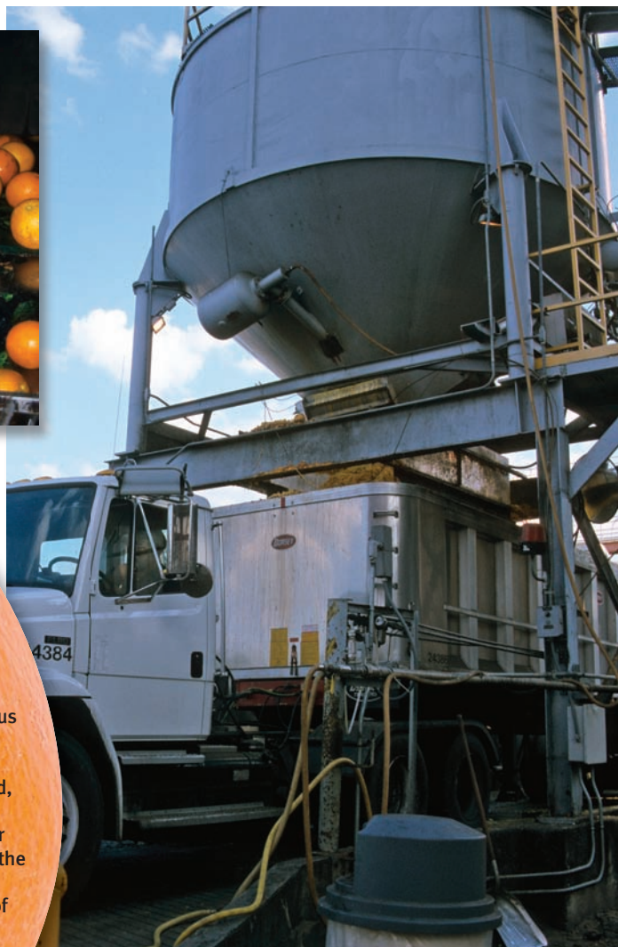
► Once the Florida's Natural facility peels the fruit and the juice is extracted, the seeds, peels, rags and pulp — about 40%-50% of a typical fruit's weight — are placed in a bin where the conversion from waste material to livestock feed begins.
