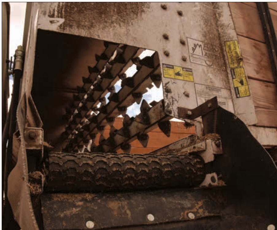
► Prior to using a TMR mixer, Eloy Mendoza of Broken Arrow Cattle was using this grinder/bale processor truck to try to feed a mixed ration to his cattle. Even after premixing the feed and pushing it through the roller blades, the cattle were still able to sort the feed.
