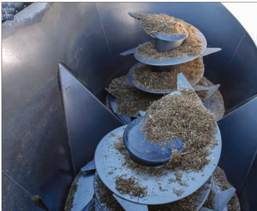
► In this TMR mixer, two vertical screws work in conjunction to mix and process long-stem hay, corn silage, straw and ground wheat. TMR mixers make a consistent ration that reduces the animal’s ability to sort when eating.
