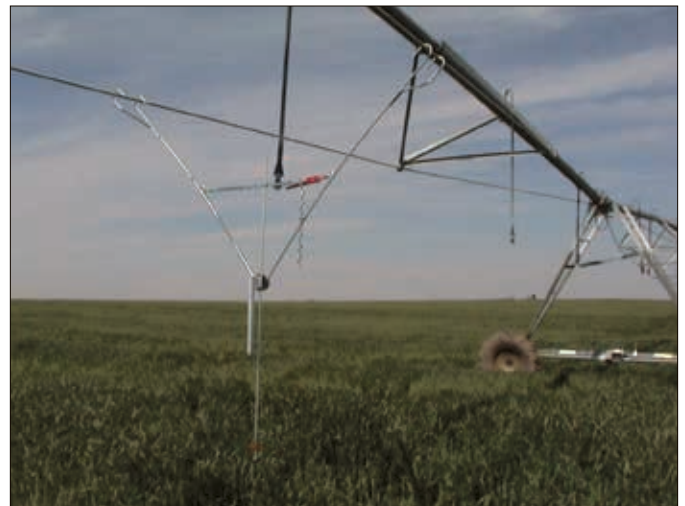
►The truss rod hanger is attached to the truss rods between each tower. Depending on the topography of the soil, as many as are needed to stabilize the wire can be used.
