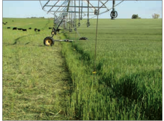
►“[The wire] can grow or it can shrink with the pivot as it moves through the field without it getting too much stress and breaking or drooping down too low and getting snagged,” explains Gross.
