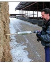
a heat-treated serrated tip and chambered extraction slot. The cores from this sampler are emptied directly into a bucket or sample bag.
