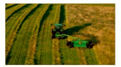
and faster dry down with less field loss, the new mower-conditioners have steel-roll conditioning systems. The two models can be matched with 125 hp or higher tractors for optimal harvesting performance.
