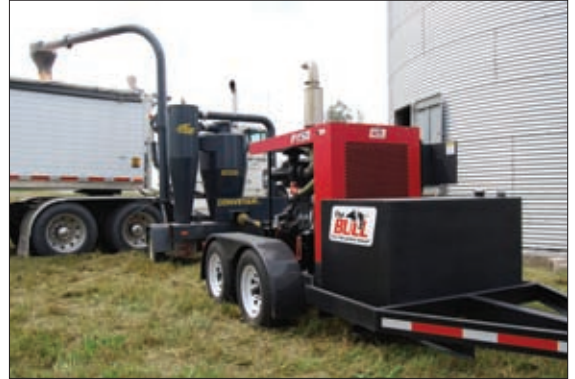
▶ "The Bull" mobile power takeoff (PTO) power source.
