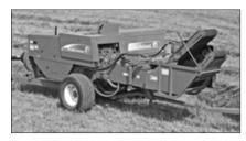
easier maintenance, according to the release. The knoter gear drive has been redesigned to make it simple to replace the pickup belt, and the oil pump has been relocated for easier service access.
