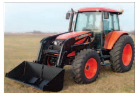
► Westendorf TA-26 Plus loader mounted on a Kubota M108S tractor
