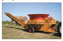
With the hammermill moved to the rear of the tub, it allows for the use of twin 12-in. by 4-ft.-6-in. dual belly augers that provide for faster discharge. A 90° tub tilt was installed for easy access to the hammermill for maintenance and service.
