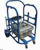
This rechargeable power supply can be charged from standard 120-volt outlets or explosion-proof outlets, and when paired with the company's EHL-LED explosion-proof LED hand lamp, can run four lamps for up to 21 hours on a single charge. The four receptacles on this unit are explosion-proof twist-lock designs rated at 20 amps and accept Larson Electronics' own EPP-15A or EPP-20 plugs or Crouse Hind™ ENP general-purpose plugs.
