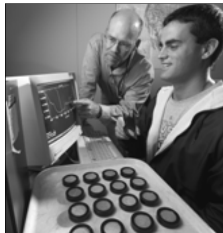
► Northup (left) and technician Kory Bollinger use near-infrared reflectance spectroscopy to develop databases that will allow forage quality to be rapidly predicted.
