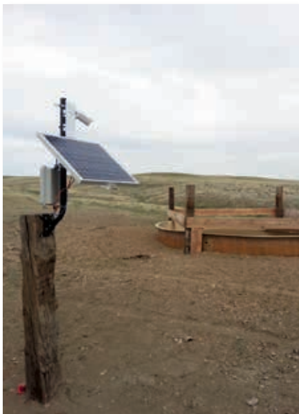
► A camera mounted on a post near a stock tank sent a video feed by directional antenna to an omnidirectional antenna located at the rented ranch’s building site. From that “hub,” video images were transmitted to Rodney Becker’s home ranch.
