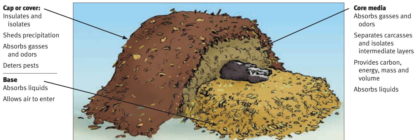
Fig. 1: Cross-section of carcass compost pile layers
