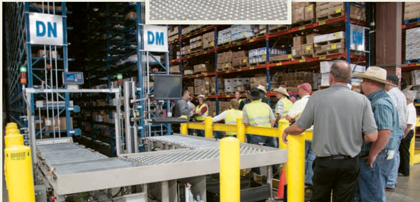
► Below & right: The mini loader, an automated robot that moves up and down the aisles on tracks, automatically selects items that will soon be needed for orders and places them on lower shelves. Once the items are in place, orders are then assembled.
