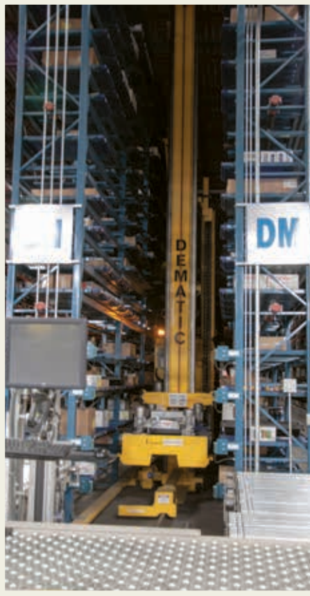
► Below & right: The mini loader, an automated robot that moves up and down the aisles on tracks, automatically selects items that will soon be needed for orders and places them on lower shelves. Once the items are in place, orders are then assembled.
