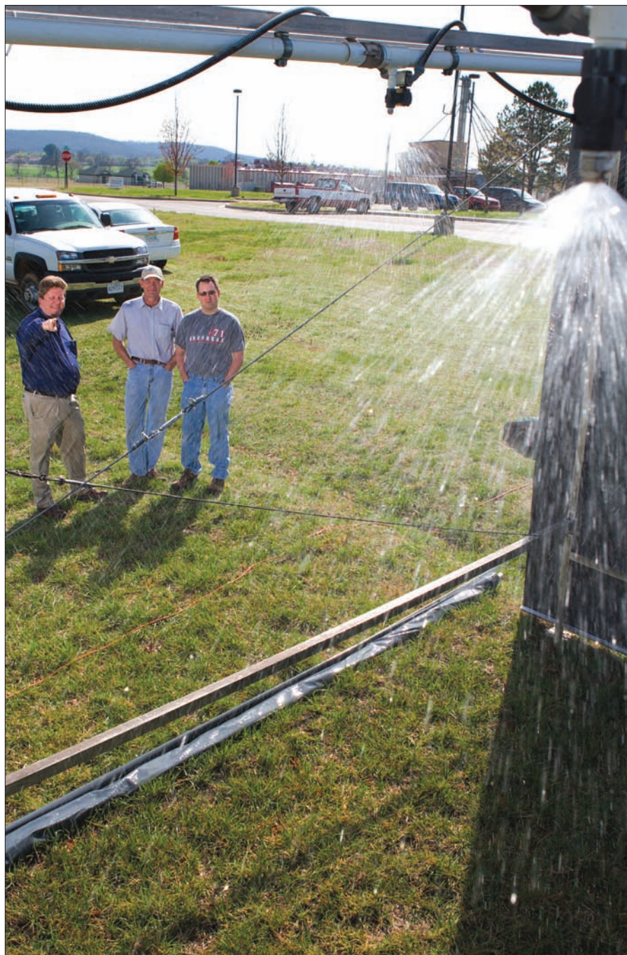
► ARS and University of Arkansas scientists conduct a rainfall simulation to determine the long-term effect of alum-treated poultry litter on aluminum and phosphorus runoff.
