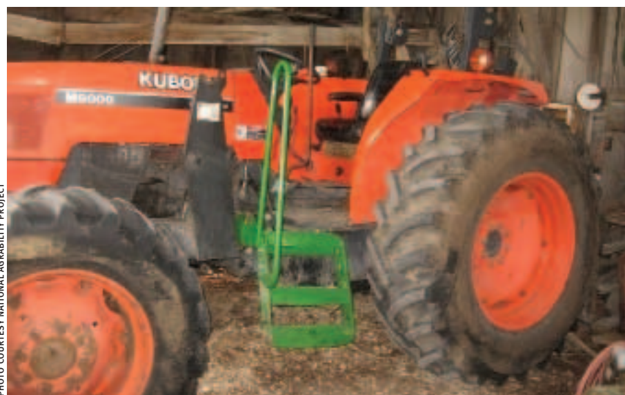
► This set of add-on tractor steps with handrail provides an example of the problem-solving inventions included in the AgrAbility Toolbox.
