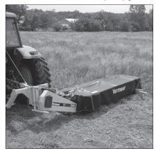
boxed section gussets. Increased cast material along the leading edge of the bar helps extend the life of the bar; increased reinforcement and support on the end of the frame also allows operators to cut closer to fencelines.
