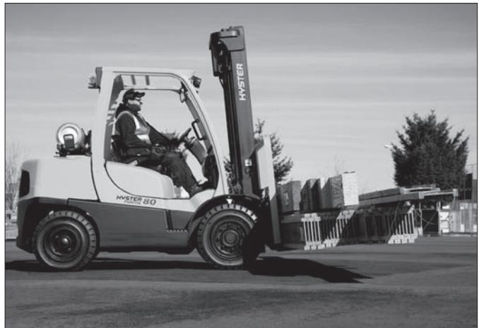
The new line, which covers a capacity range of 2,000 pounds (lb.) to 15,500 lb., offers both cushion and pneumatic tire classes, with multiple engine choices consisting of gas, LP and diesel. The different configurations simplify lift truck purchases with a tiered system of preconfigured engine-transmission bundles.
