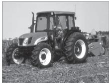
available with a choice of two-wheel, four-wheel or the company's SuperSteer<sup>™</sup> axle. There are additional transmission options, a new independent 540/1000 rpm shiftable power takeoff (PTO) option, a
