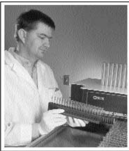
► Technician George Perry conducts a radioimmunoassay to measure progesterone concentration in serum samples from cows that ovulated different-sized follicles.
