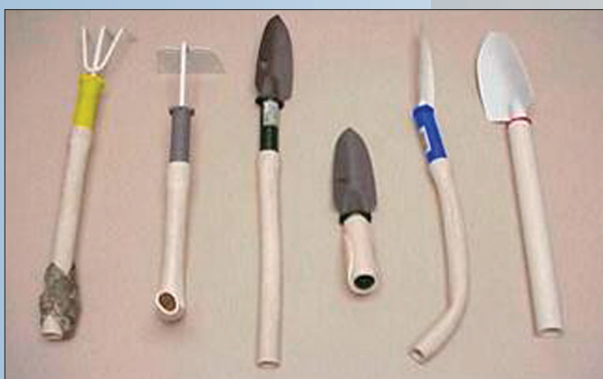
► Extending a tool's handle can improve leverage, making it easier to use.
