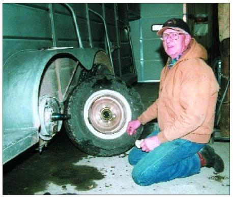
► Above: With 25 years of professional experience in maintaining and repairing virtually all makes of trailers, Vern Oatman recommends careful attention to the basics, including brakes, wheel bearings, tire pressure and lights.
