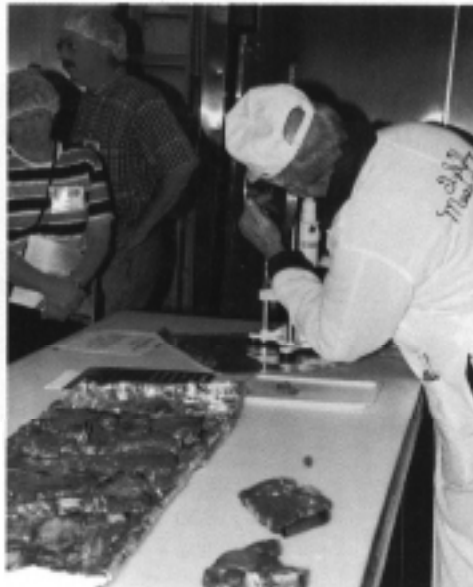
Monday afternoon, National Conference attendees toured the Iowa State University (ISU) animal science department. During the tour, ISU faculty demonstrated a Warner-Bratzler shear force test.
