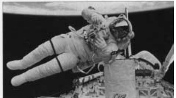
Astronaut Mark Lee tests the new Simplified Aid for EVA Rescue (SAFER) system 130 nautical miles above Earth
