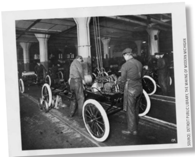
Ford Motor Company Model T assembly line, 1913.
