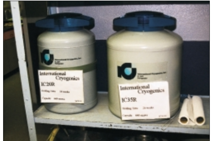
Double-walled, liquid-nitrogen tanks can be purchased by breeders to store semen. These tanks should be checked every 15 weeks for nitrogen levels. The nitrogen level in the tank should never get below two-thirds of an inch.
