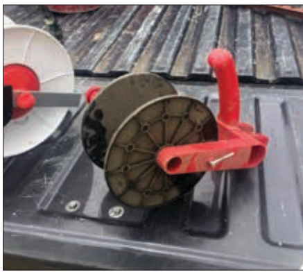
▶ Gerrish uses these reels for running wire in between two temporary fences. They will hold up to 600 ft. of polybraid. He braces both ends with his O'Brien post trick and hangs these beside the brace.
