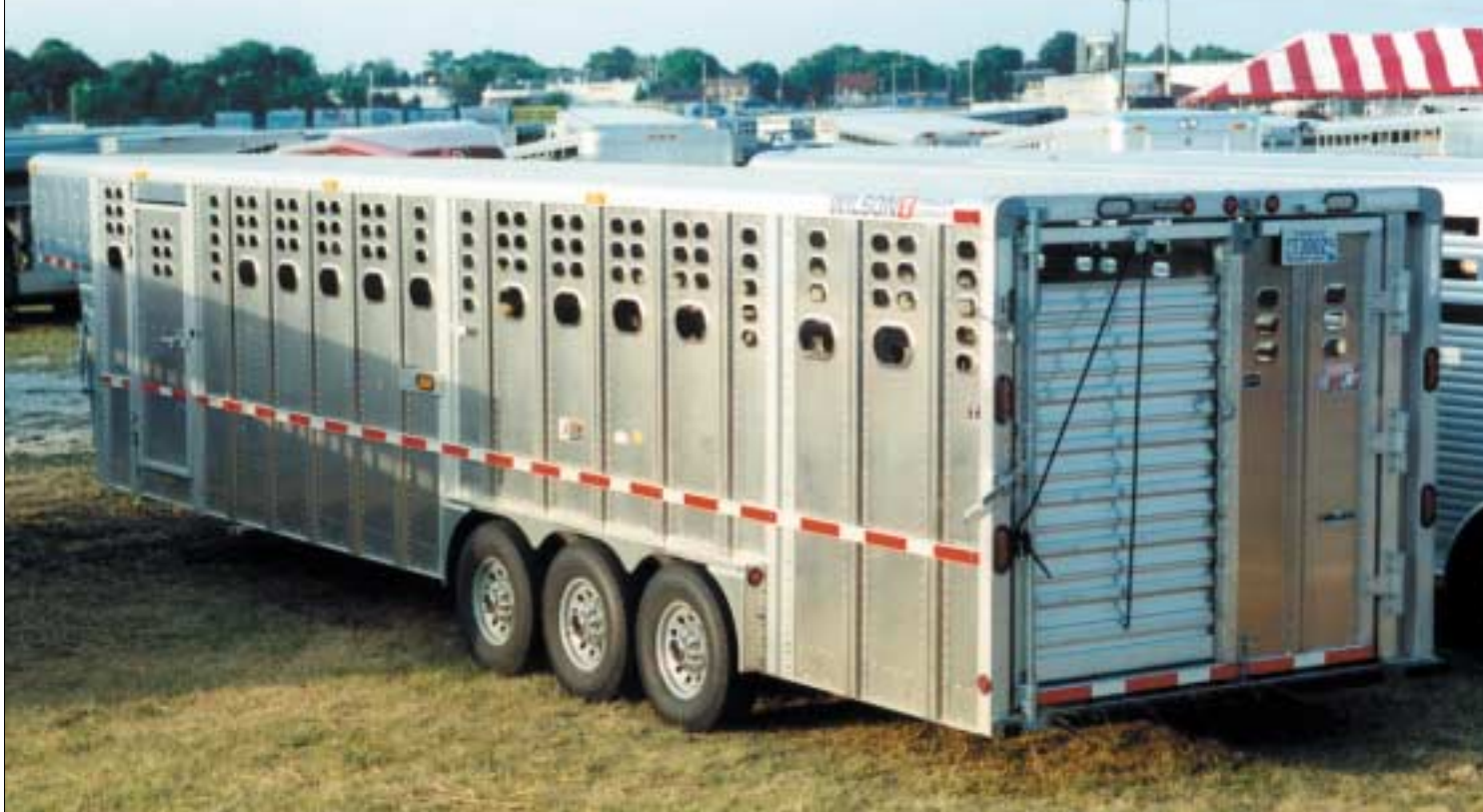
► There are many different slat patterns from which to choose when shopping for a trailer. If the trailer will be used during extremely cold weather, a buyer should be concerned about ease of closing or blocking openings to control airflow.
