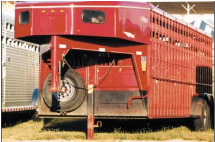
►A spray-on gravel-guard coating often is used to protect the front and fenders of trailers used on gravel roads. Some trailer owners also use the coating to protect the inside of steel trailers.
