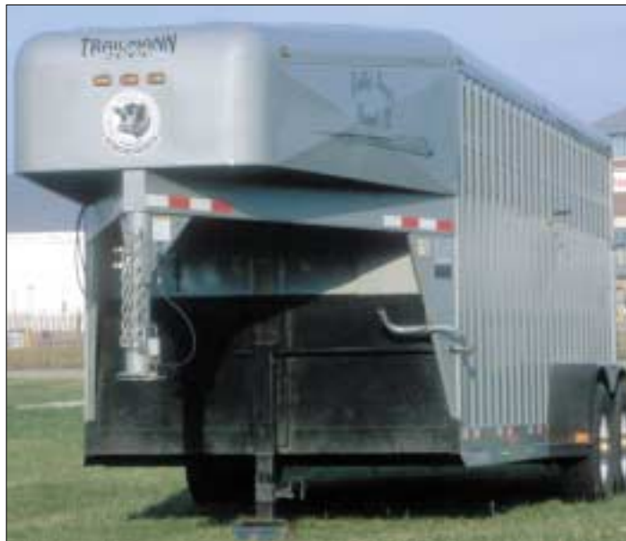
►Left: Consider aerodynamics when selecting a trailer. The nose shape and height of the trailer are key factors in wind resistance.
