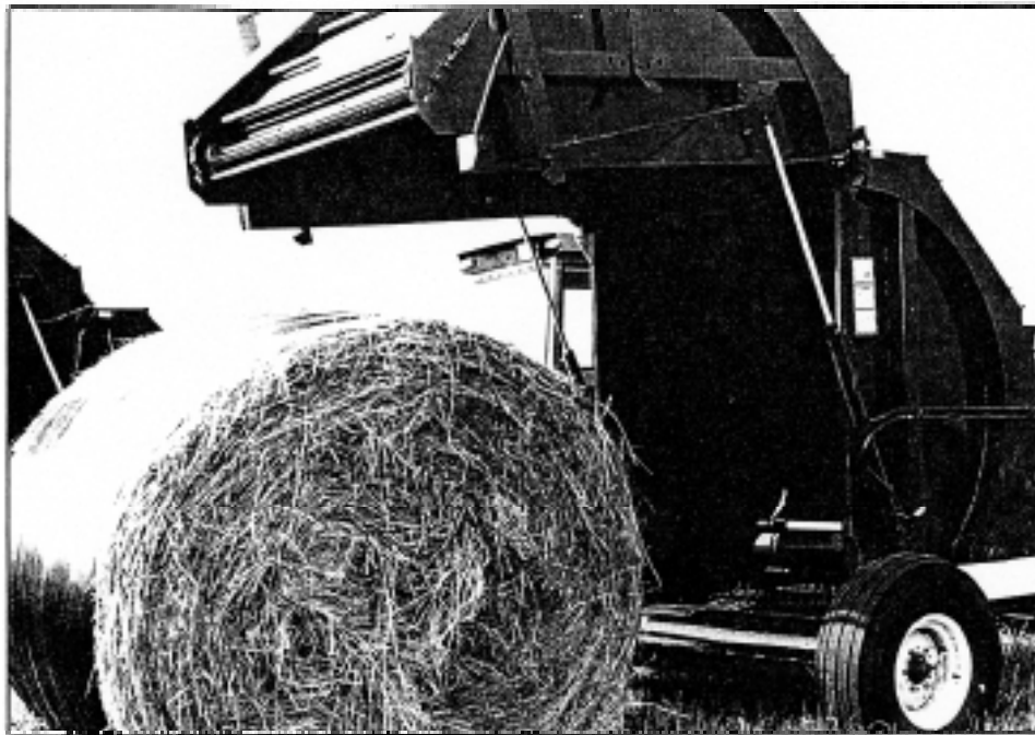
This M&W 1800 baler wraps bates with 1.5 mil plastic before leaving the chamber. M&W recommends bates be wrapped at least three times for the plasticsleeve to be effective.
