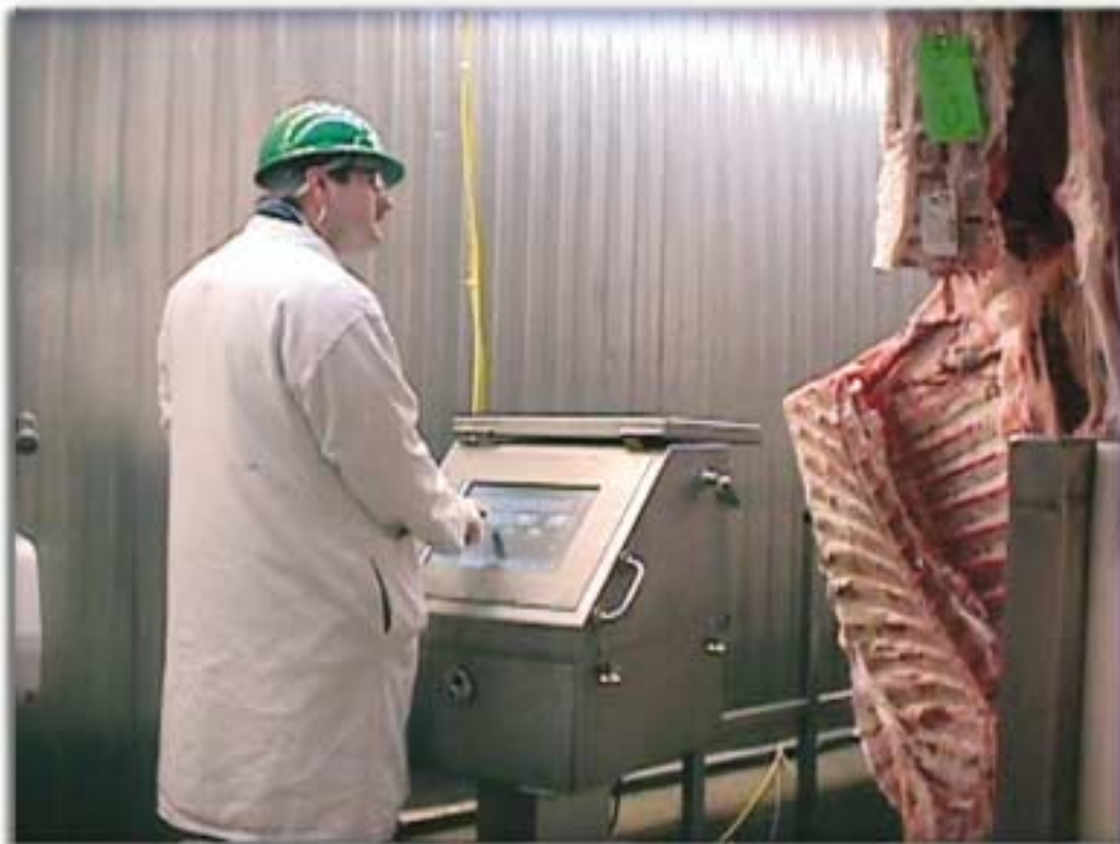
The Computer Vision System (CVS) is a two-camera arrangement capable of capturing and channeling carcass information through different software modules. It was recently approved by the U.S. Department of Agriculture (USDA) to help its graders assign more accurate yield grades.
