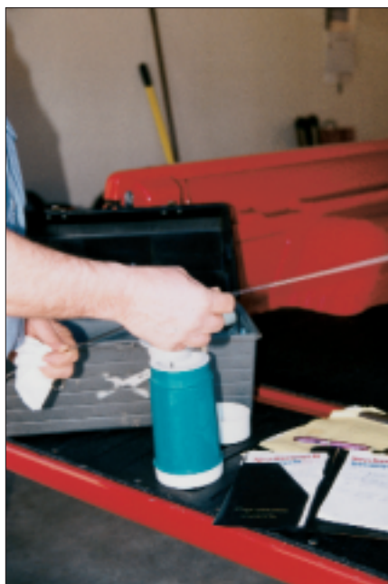
There are several types of syringes (or guns) on the market, including the spiral syringe and the "O-ring" syringe. Each has a uniquely suited disposable sheath style.
