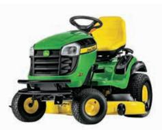
The 100 Series has side-by-side forward and reverse pedals and a redesigned cut-height lever and a larger reverse implement option (RIO) switch. Lastly, the ReadyStart<sup>®</sup>
