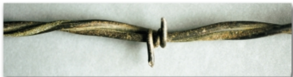
This forerunner of the wire design commonly seen today was patented in 1874 by Joseph Glidden. With two twisted strands and two-point barbs around one strand, this design was declared the winner in the legal fight over barbed-wire patents. Today collectors value this wire at about 24¢/18-inch piece.
