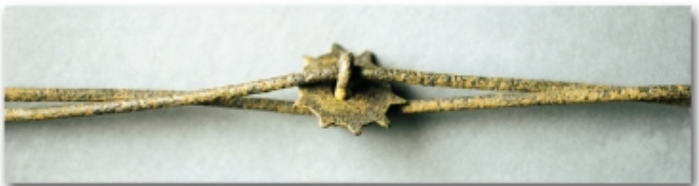
A twisted two-strand wire with 10-point spur rowel barbs made of sheet metal was patented in 1887 by Chester Hodge of Beloit, Wis. Its approximate value is $5.
