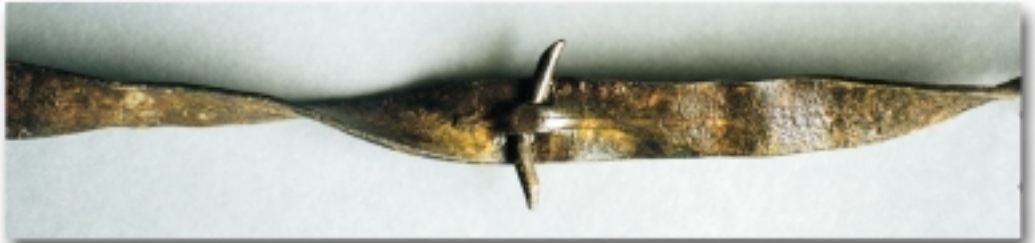
This 1882 split-ribbon variation by Illinois inventor Andrew Upham featured a twisted sheet-metal ribbon with two-point wire barbs set in slits that were cut in the ribbon. Its approximate value is $20/collector sample.
