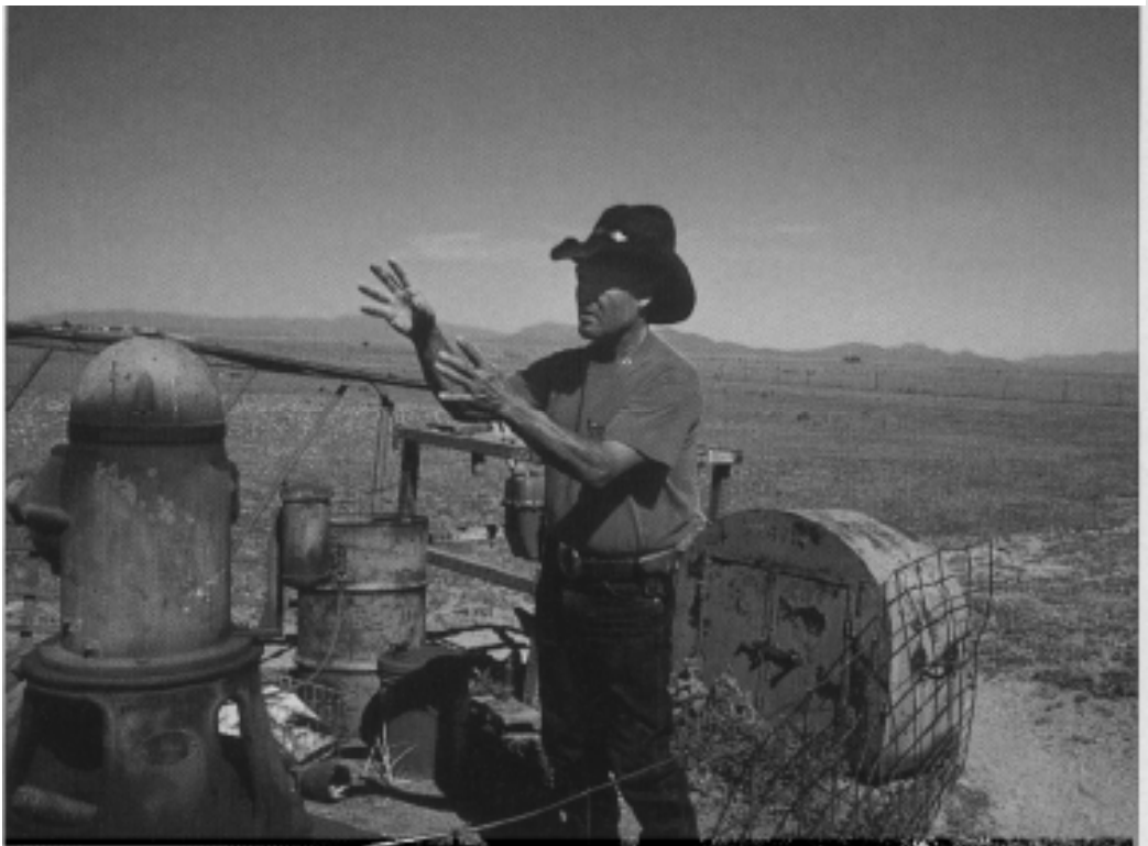
Irrigation is a necessity on the Montoya Ranch, where annual precipitation averages 7.5 inches. Fidel's irrigation well is 100 feet deep and produces 4,200 gallons of water per minute when powered by a 454 engine.
