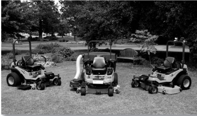
mowing on slopes. For safety, the power take-off (PTO) clutch is equipped with an internal brake to stop mower blades quickly after disengagement.
