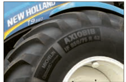
► The Michelin AxioBib IF850/75R42 prototype, the largest tire in the company's lineup.
