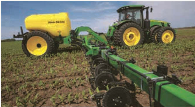
► John Deere 2510L liquid-fertilizer applicator
